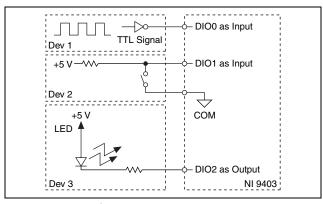
Figure 2. Connecting Digital Devices to the NI 9403
